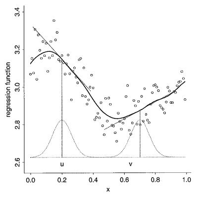
Figure 3.23 Local linear scatterplot smooth (solid curve) based on 100 simulated observations (represented by circles). The dotted curves are the kernel weights and cubic fits at the points u and v.
